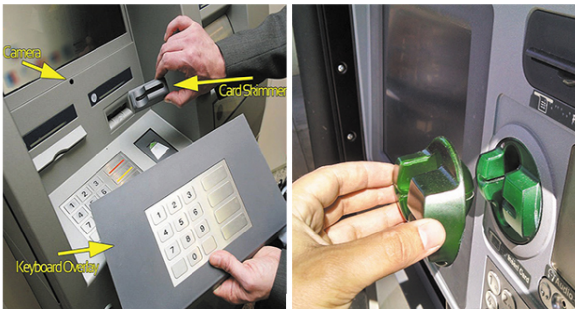
Skimming devices, which steal information from an ATM card's magnetic stripe, are difficult to detect.
